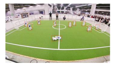
Fig. 5. Example of detected robots in a video recorded with a GoPro camera at the RoboCup 2018 in Montreal/Canada.
