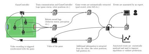
Fig. 1. Overview over the data flow of the implemented data processing ecosystem.
