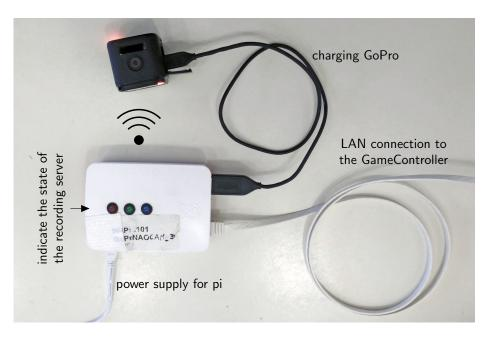
**Fig. 2.** System for automatic recording of synchronized RoboCup videos. The recording server is based on raspberry pi with the colored indicator LEDs. The GoPro is charged via USB from the raspberry. A LAN cable connects the pi to the GameController network. The Recording server sends commands to the GoPro via WiFi.
