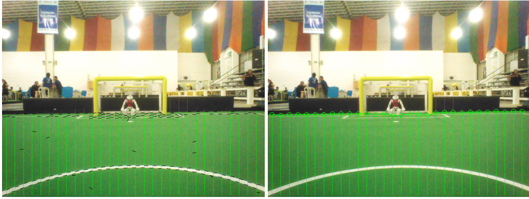
Figure 4.4: With top to down scanlines [green lines] the edges of possible field lines [black lines] including their orientation are detected (left) and the last field colored points are assumed as endpoints of the field [green circles] (right).
