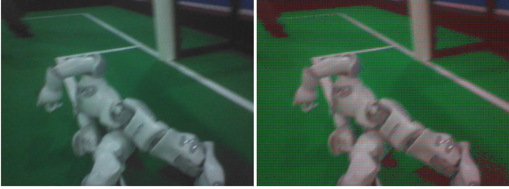
Figure 4.2: (left) Example image from the Iran Open 2015. (right) Pixels classified as green are marked green; pixels with too low chroma marked red;
