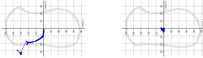
**Fig. 3.** Robot changes from standing by double feet to the standing on one leg, i.e., prepare for the kick. The left figure shows that center of mass jumps out of support polygon without stabilizer; the center of mass is kept in the center of support polygon with stabilizer in the right figure.
