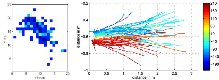
**Fig. 6.** The kick is performed with the same direction but from random positions: (left) positions of the ball. The color indicates the number of kicks from the according position (the greener, the more); (right) observed trajectories of the ball for each kick position (respective colors);
