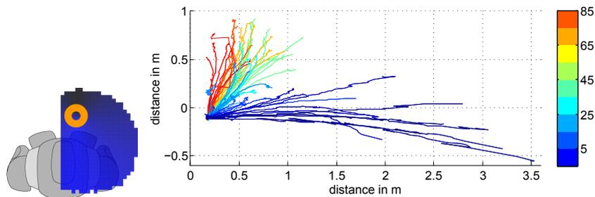
**Fig. 4.** The kick is performed with the same starting position of the ball but in different directions: (left) position of the ball and the reachability grid; (right) observed trajectories of the ball for each kick direction (respective colors);
