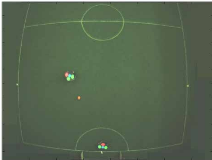
Fig. 2. Barrel distortion of the field with a 4.2 mm lens
