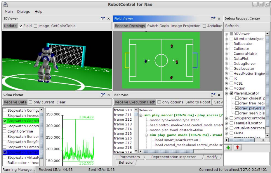
Fig. 3. The RobotControl program contains different dialogs. In this figure, the left top dialog is the 3D viewer, which is used to visualize the current state of robot; the left bottom dialog plots some data; the middle top dialog draws the field view; the middle bottom shows the behavior tree; and the right one is the debug request dialog which can enable/disable debug functionalities.
