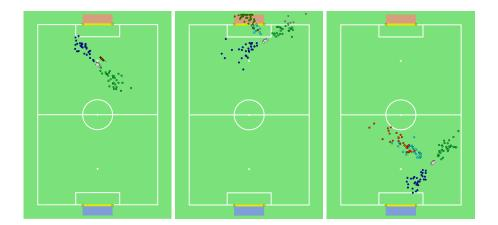
Fig. 3. Three examples for kick simulations. Each possible kick direction is simulated with 30 samples (different colors correspond to different kicks). Left: the short and long kicks are shortened due to collision with an obstacle. Middle: long kick is selected as the best action since it has the most samples result in a goal. Right: the best action is sidekick to the right – the other kicks are more likely to end up in a dangerous position for the own goal according to the potential field.
