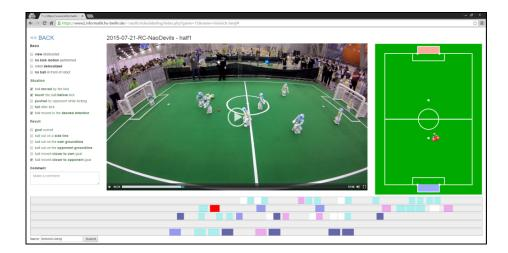
**Fig. 6.** Illustration of the labeling interface used to collect data regarding the quality of the kicks. At the bottom are time lines for each of the robots. Different actions are represented by buttons on the time line with different colors. On the right the robots estimated state is visualized, i.e., estimation of its position, ball model and obstacles. On the left are three categories of labels capturing the quality of the action.
