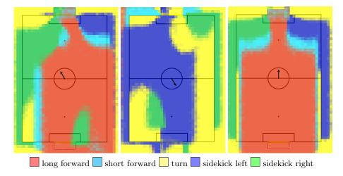
**Fig. 5.** Resulting decisions based on different positions of the ball on the field and three different orientations of the robot. Different colors correspond to differnt decisions. The orientation of the robot is indicated by the arrow. Own goal is at the bottom, opponent at the top.
